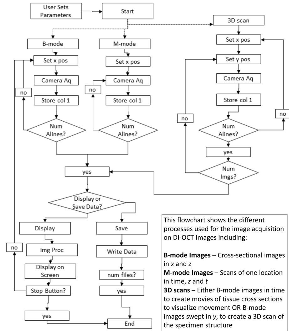
This flowchart shows the different processes used for the image acquisition on DI-OCT Images including:
