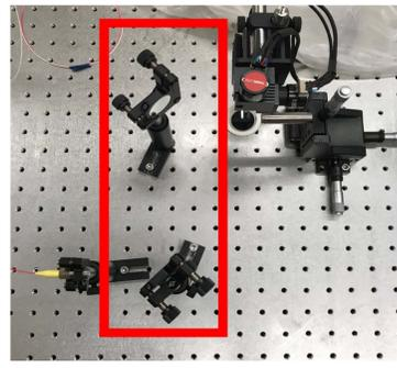
**Left** – Periscope used to steer the laser beam to the sample for imaging. This enabled the precise alignment required to couple laser energy scattered from the sample back into the interferometer.
