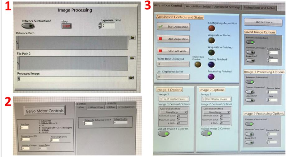
Above are two different GUIs for the DI-OCT System GUI; Images 1 saves images to the computer and 2 control the image scanning technique, Image 2 shows a GUI of a similar systems showing what the end product for DI-OCT should look like. Ultimately, the sub-GUIs such as those in Images 1 and 2 will be combined into a master GUI such as that in Image 3.
