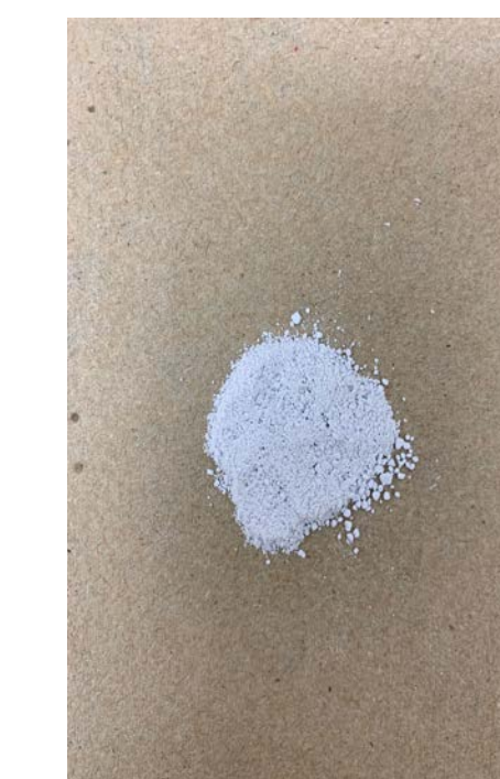
Figure 11. Preliminary process used to grind up PVC into powder that would be of consumable size. PVC cards (~2x4 in.) were put into a blender, followed by a coffee grinder. The grinding of the PVC particulates generated a powder on the lid of the coffee grinder. A plastic scooper was then used to scrap the powder off the sides of the lid (Figure 12).
