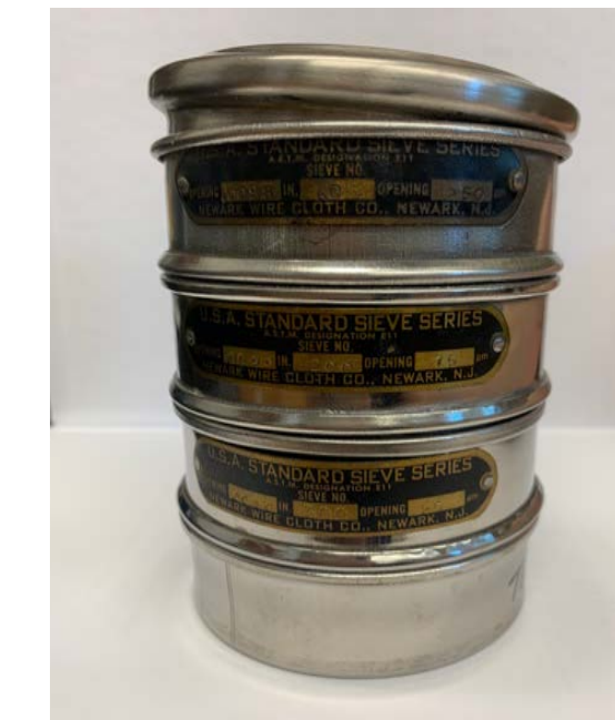
Figure 4. Metal sieves for particulate size determination
