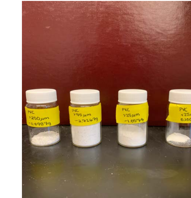
Figure 5. Separated particulates based on sieving fractionation
