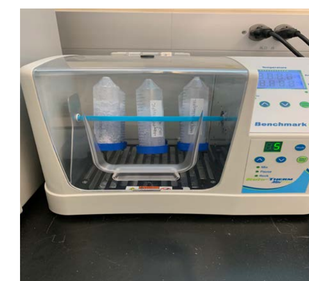
Figure 6. Incubation Rotator. Continuously mixed samples at 15 rpm in 37°C
