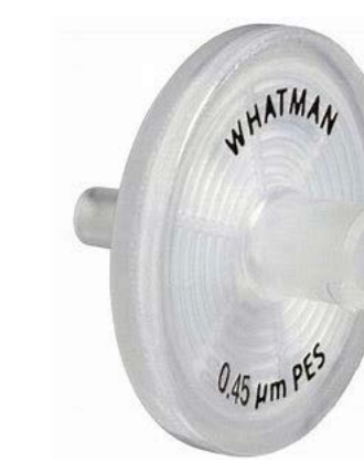
Figure 7. Syringe filter used for sample syringe filtration
